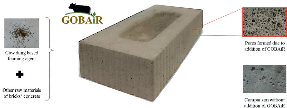
Figure 1. Light weight block developed using GOBAiR
